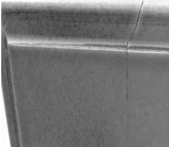
Above: Photo of joint separation at door edge
